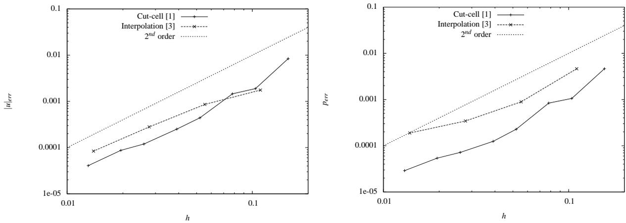
**Figure 2:** Error decrease with the spatial resolution. Left: velocity error. Right: pressure error.
