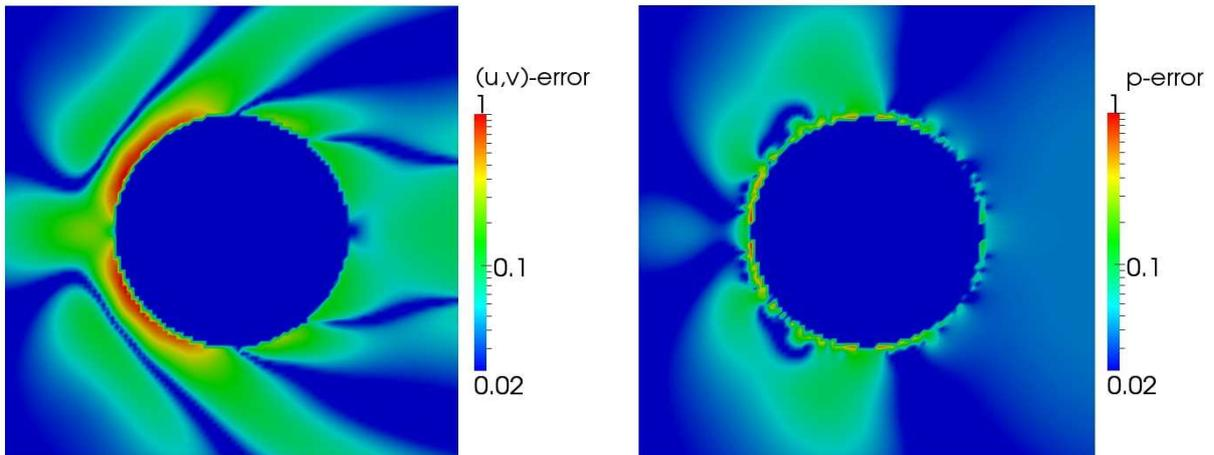
**Figure 3:** Maps of normalized error at the resolution  $1024^2$  in the subdomain  $[-D, D]^2$ . Left: velocity error. Right: pressure error.
