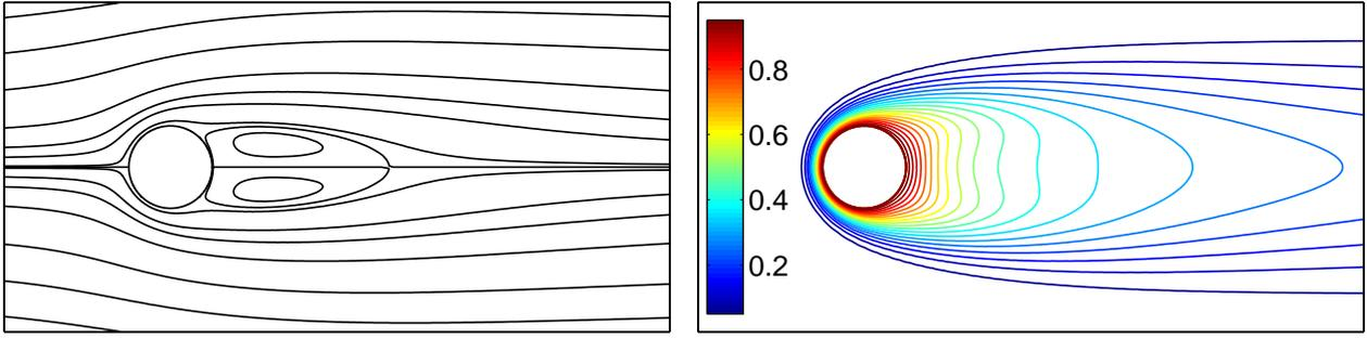
**Figure 1:** Streamlines (left) and passive scalar isocontours (right) for the flow over a circular cylinder at  $Re = 40$  and  $Pe = 40$  (reference solutions).
